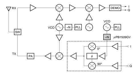
This block diagram schematically shows the  $\mu$ PB1509GV's location in one of the example application system. The other applications are also acceptable for divider use.
